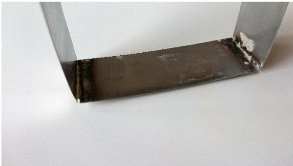
Figure 27: Broken cutting mold (2).
