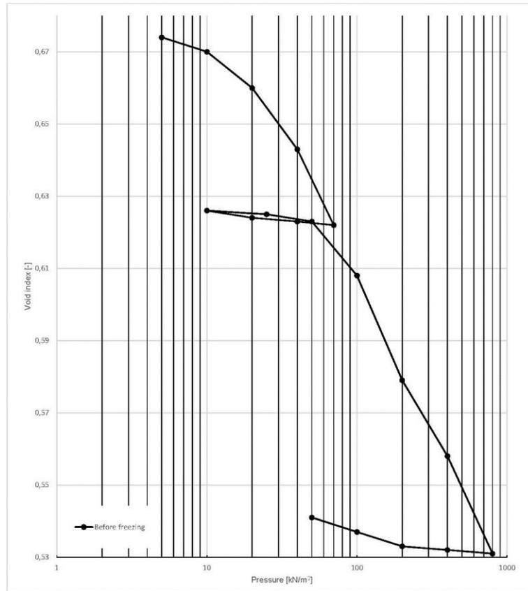
Figure 19: Initial oedometric curve.
