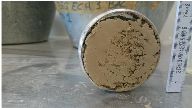
Figure 38: Specimen 3 with voids caused by ice lens.
