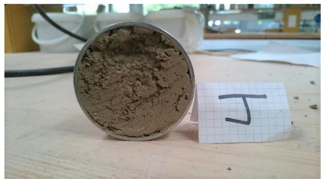
Figure 42: Sample before CRS test 3.
