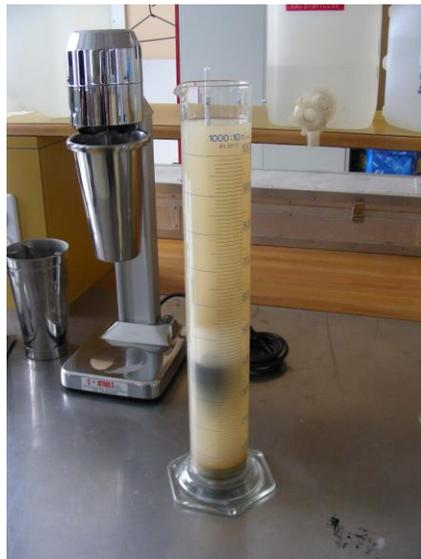
Figure 3: Sedimentometry.
